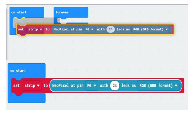
Move the "set strip" block next to the "on start" block until you see a yellow margin appear under "on start". Release the click and the "set strip" block will fall in correctly.
