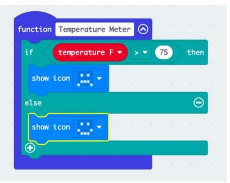
This function tells micro:bit to display a sad face when temperature is above 75 degrees, so that you know it's time to blow some wind to your plants.
