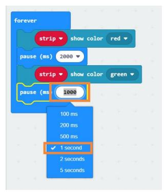
For this step, place one "pause" block after each "strip show color" block, then open the drop down menus to define how long you want the pauses to last.
